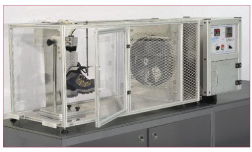
This machine has been developed to assess the thermal and sweat management performance of complete footwear by measuring thermal insulation, moisture absorption and breathability properties, tested in conjunction with hose.
