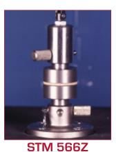
The transverse through thickness tensile strength through thickness of sheet materials, usually called the 'AZ tensile test', is measured using this device.
