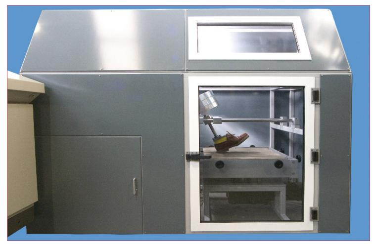
SATRA's Pedatron biomechanical abrasion tester provides an accelerated wear simulation under realistic conditions.
