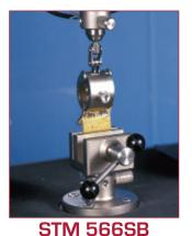
This specially shaped 'C' clamp is normally used in the peel strength testing of footwear sole to upper. It can also be used as a general purpose clamp.
