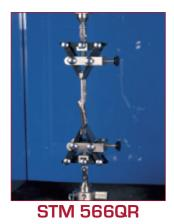
This is a unique self locking jaw with a quick release action, which can be used as a general purpose clamp for many duties.
