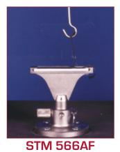
This is used for testing the strength of adhesion of the finish to the leather or synthetic material. It consists of a hook attached to one jaw and a sample holder to the other.
