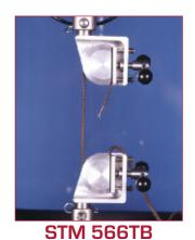
These SATRA thread bollards are used to determine the breaking load of threads and laces.
