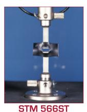
Often called the 'Baumann tear test', this is the industry standard for testing the tear strength of leather.
