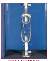
**STM 566WT** Supplied as a pair, the top-line bollards are used to determine breaking force and extension at break of whole shoe toplines.
