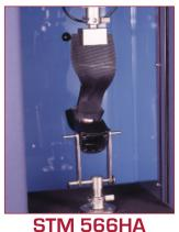
This is used to measure the strength of attachment of heel to shoe.
