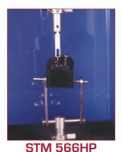
This test was developed to assess the strength required to pull a nail from the heel of footwear.
