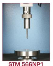
This tests a whole sole unit, complete with protective midsole, for nail penetration.
