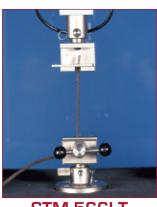
**STM 566LT** This is used to assess the attachment strength of the shoelace tag to the lace.
