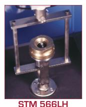
With this attachment footwear lastometer tests can be carried out to check the burst or crack strength.
