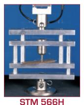
This attachment is used to determine the strength of footwear insole board, particularly in the seat region.
